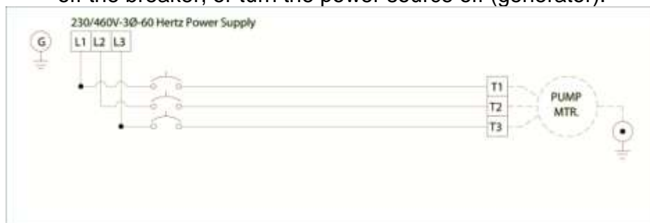
Typical 3 phase manual control 1
