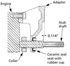
Figure 1 – Mechanical Seal Replacement
