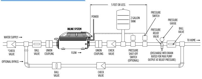
NOTE: These optional components are shown in a typical installation diagram. They should be used at the installer's discretion as required for particular applications.
