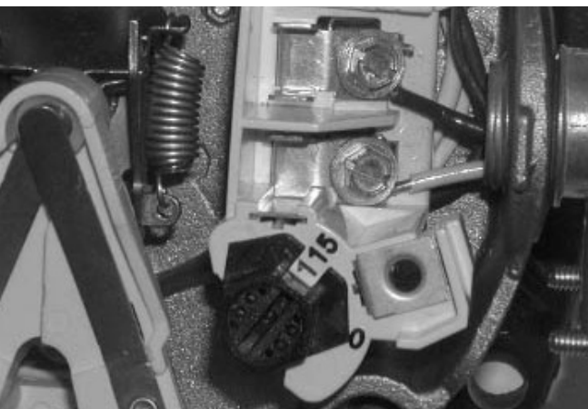
Figure 4: Motor Set for 115 Volt Operation
