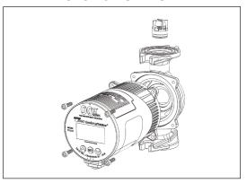
To rotate the casing, remove the 4 motor screws and spin the casing to the desired flow direction. Reattach the 4 screws  $\{\S_{32}^{u}\ allens$  wrench required). Be sure body gasket is seated evenly to prevent leakage. Tighten motor screws to 34-42 inlbs torque.
