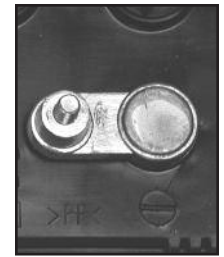
NEGATIVE POST HAS SMALLER DIAMETER
