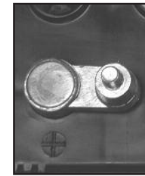
POSITIVE POST HAS LARGER DIAMETER
