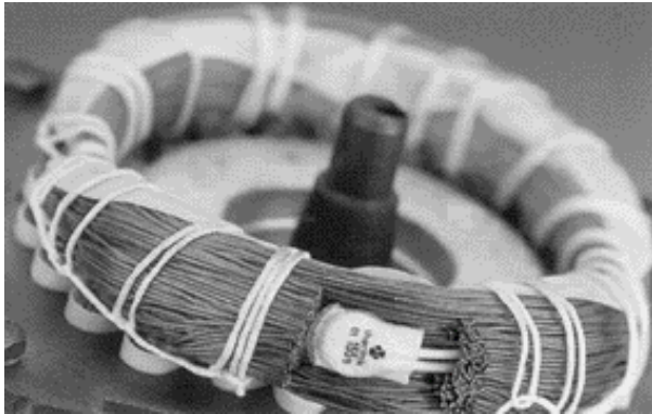
Thermal switch incorporated in winding
