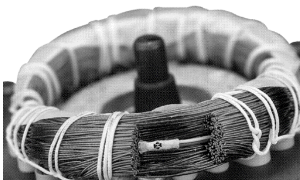
PTC sensor incorporated in winding
