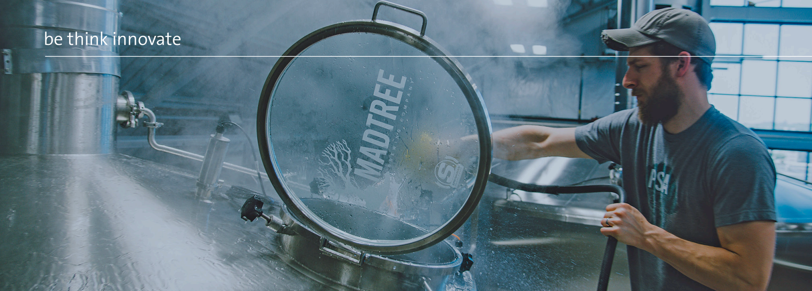
Above: Director of Brewing Operations, Matt Rowe, sprays out the mash / lauter tun on MadTree's 126 BBL production brewhouse during a brew day.
