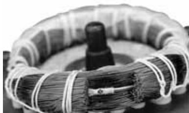
Fig. 40 PTC sensor incorporated in windings
