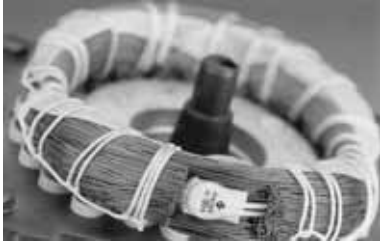
Fig. 42 Thermal switch incorporated in windings
