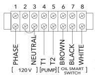
\* For 240V, remove jumper and supply power to terminals 1 and 2, with neutral on 3.
