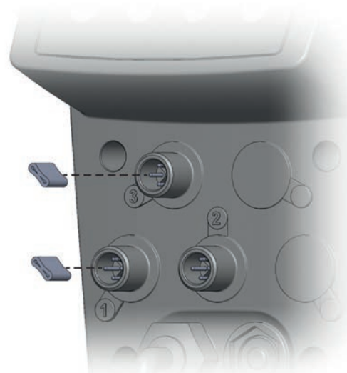
Fig. 16: Conductive rubber hoses in the connections 1 and 3 of the MAGDOS LA/LD
