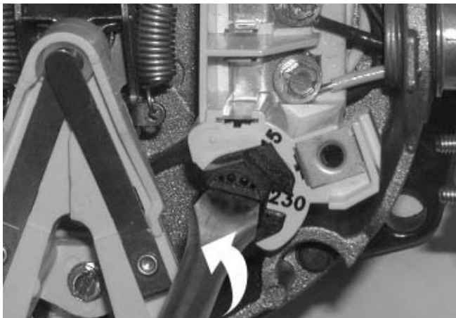
Figure 3: Changing the Voltage Setting
