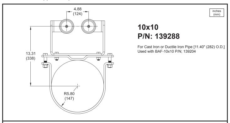
The intermediate guide rail support is required for every 13 feet (14m) of guide rail.
