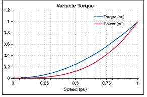
Common variable torque loads include pumps, fans, and compressors. The value of load inertia that can successfully be synchronized varies by frame size and is typically lower than for a comparable NEMA induction motor. The inertia synchronization capability for each stock rating can be found in Table 1. For loads where the required torque exceeds the variable torque profile or the load inertia is in excess of the value listed, contact your local Baldor District office for proper sizing.
