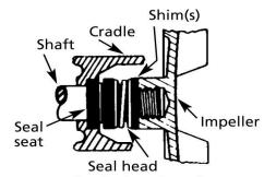
Figure 1 - Mechanical Seal Replacement
