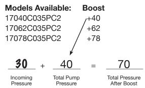
Based on this example, the recommended model for this application is the 17040C035PC2.
