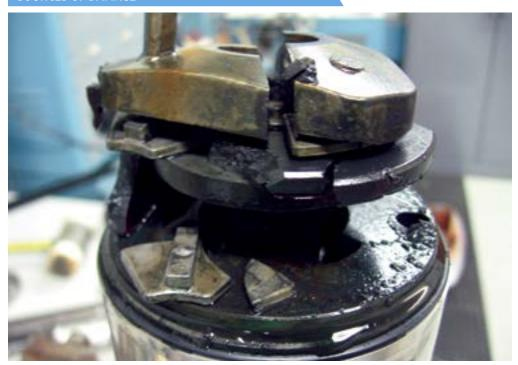
Broken Thrust Bearing, Support, And Thrust Pads
