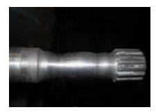
**Severely Worn Shaft** Visible
