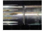
Shaft Damaged Below Spline by Improper Coupling Installation Not Warrantable
