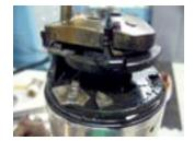
Extreme Shock Required to Fracture/Split Bearings
