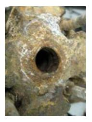
Corrosion and Rust in Prong Hole
