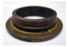
Sand Worn Shaft Slinger Bushing Visible
