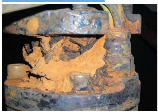
Aggressive Environment Causes Corrosion
