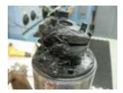
Improper Cooling and Thrust Loads
