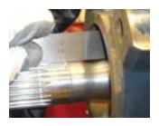
Motor Shaft Damaged by Gravel in the Pump Intake Not Warrantable
