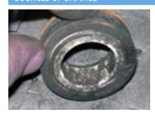
**Abrasive Covered Seal/Worn ID**Not Visible
