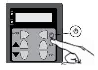
The pump starts and reaches the pressure level set at the factory (default is 60PSI). The RUN/FAULT LED will be ON and showing green. If the system pressure is equal to or higher than the factory pressure setting, the pump will be in stand-by mode (green LED ON), ready to start if the pressure decreases.
