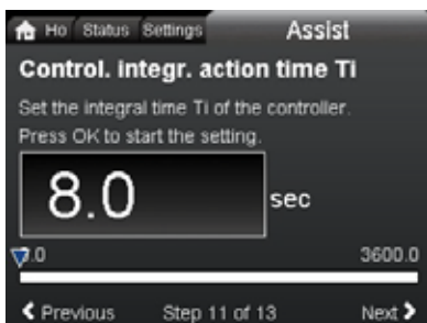
Fig. 61 "Control. integr. action time Ti"
