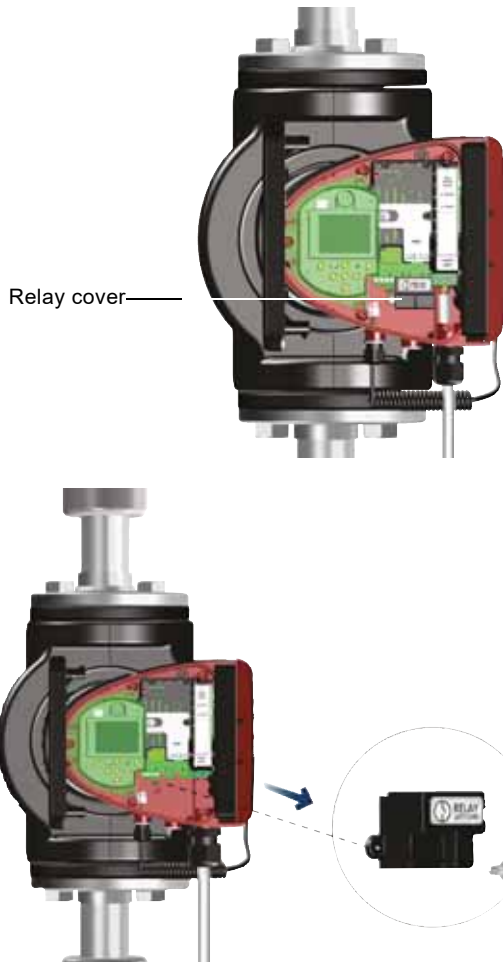
Fig. 45 Removing the relay cover
