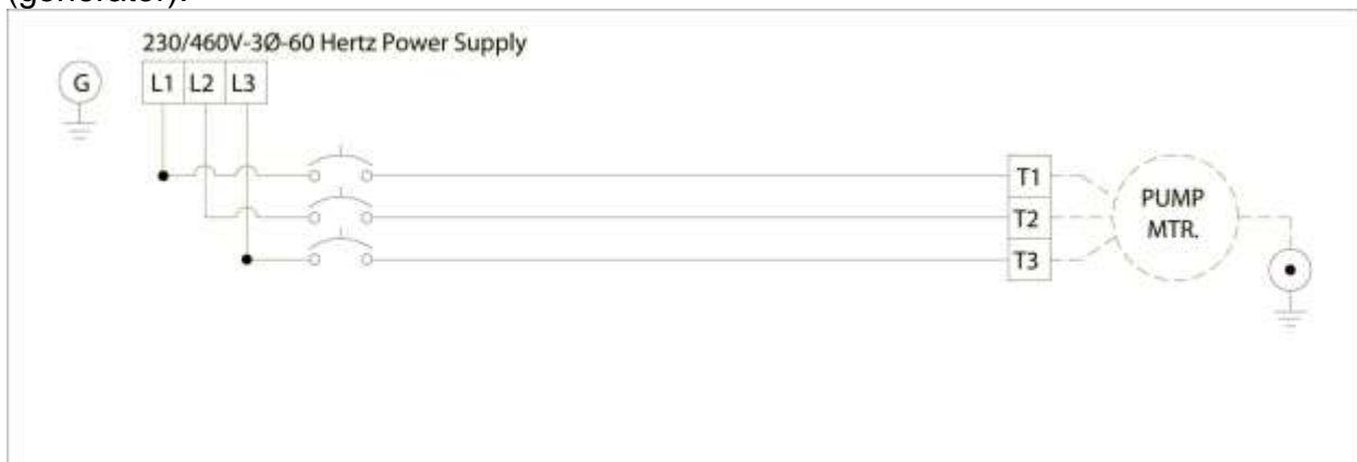
Typical 3 phase manual control 1
