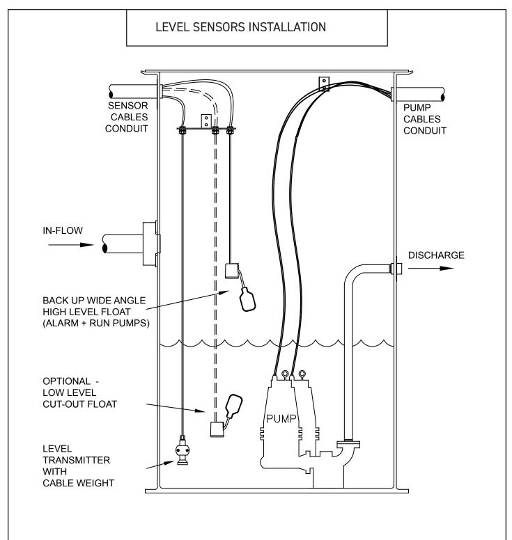
Typical transmitter (with high level float back up) setup for a duplex lift station
