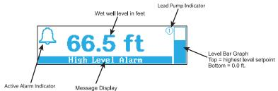
The main screen displays the set well level and any active alarms. The controller will return to the main screen automatically after 3 minutes of inactivity.
