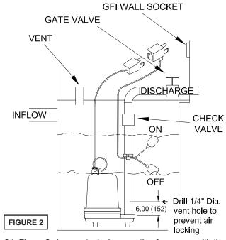
Figure 3 shows a typical connection for pumps with the wide angle float and piggy-back plug, for manual and automatic operations.
