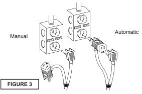
**Automatic -** Plug float cord into GFI outlet, then plug pump cord into float cord.
