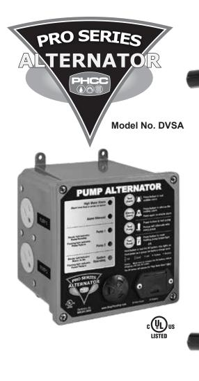
The PHCC Pro Series Pump Alternator is designed to operate two primary pumps. Every time the float switch is activated, it will automatically alternate the pump that turns on. This will prolong the life of both pumps. If one of the pumps fails to turn on, the Alternator will automatically switch to the other pump. If this occurs three times in a row, a light will start flashing indicating exactly which pump is failing.
