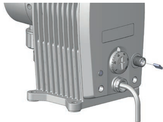
Fig. 15: Inserting the conductive rubber band
