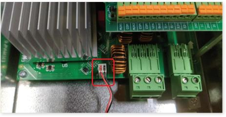
NOTE: On the 5HP models (SD3-5HP2) you will need to disconnect the four (4) CAT5 cables that connect the control board to the inverter board, remove the four (4) screws that attach the control board to the inverter board, remove the four (4) threaded standoffs from the inverter board and the two screws that hold the inverter board to the back of the enclosure. Then remove the inverter board and it's attached fan shroud revealing the 5HP's two (2) fans.
