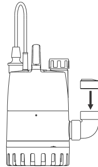
Fig. 9 Correct position of a non-return valve
