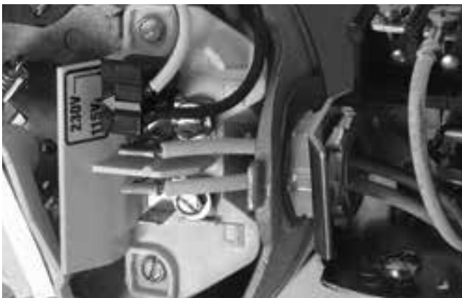
Figure 9: Voltage set to 115 volts, Plug Type
