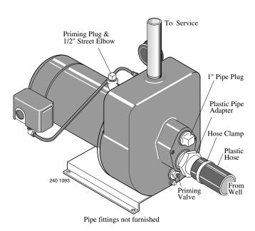
Figure 3 - Shallow Well Installation
