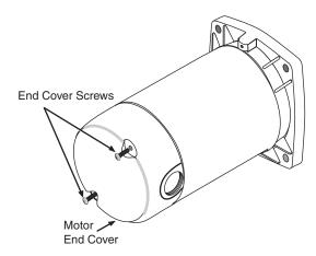
Figure 4 – Removing Motor End Cover
