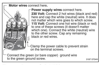
Figure 6 – Pressure Switch Wiring
