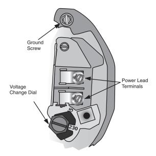
Figure 5 - Voltage set to 230 volts, Dial Type
