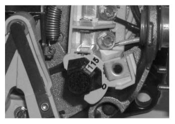
Figure 4: Motor Set for 115 Volt Operation
