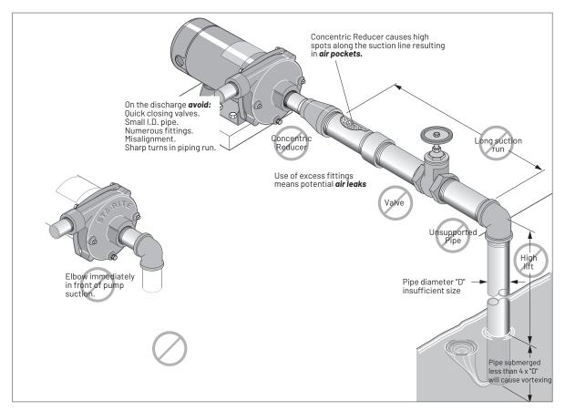
Figure 2 - Not Recommended Connections
