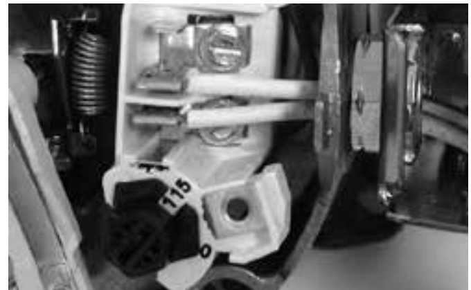
Figure 9: Voltage set to 115 volts, Dial Type
