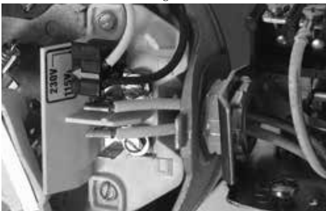
Figure 7: Voltage set to 115 volts, Plug Type
