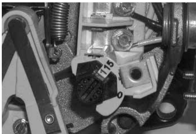
Figure 13: Motor Set for 115 Volt Operation
