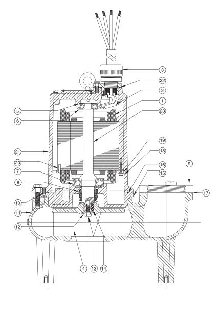
Notes: S — Parts in Seal Kit C — Parts in Carbide Seal Kit — Fill Oil to above Motor Windings
