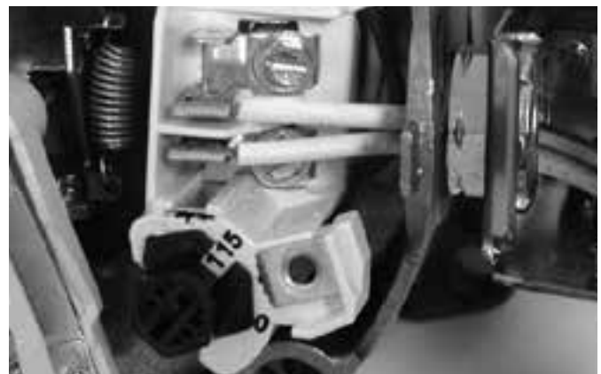
Figure 8: Voltage set to 115 V, Dial Type
