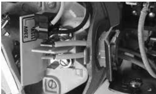
Figure 6: Voltage set to 115 V, Plug Type
