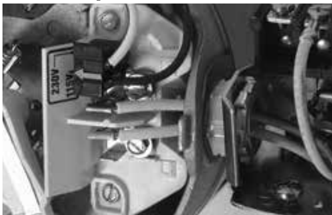
Figure 9: Voltage set to 115 V, Plug Type
