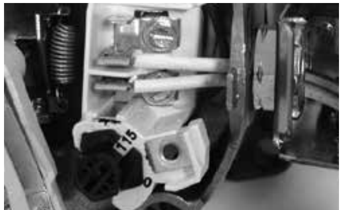
Figure 11: Voltage set to 115 V, Dial Type
